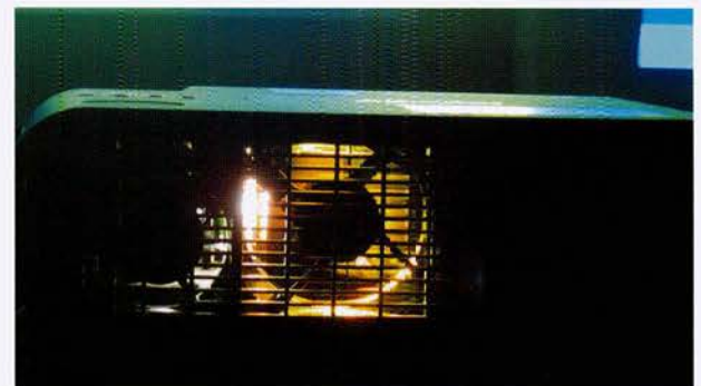
Light leaking from Mitsubishi vent
