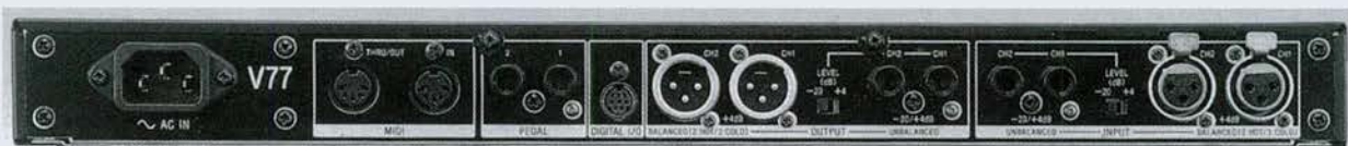
Out back, all you need. Input & output XLR's are balanced, and wired pin 2 hot as they should be.
