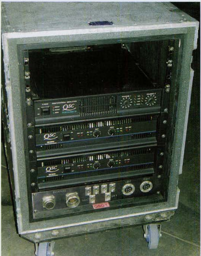
A GoLight amp rack, with neat CEEP multipin signal feed
