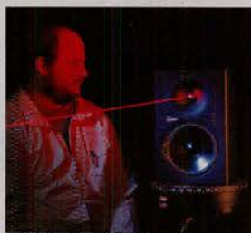
Real-time FFT laser vibrometry helped smooth and extend the HR824's treble transducer characteristics
