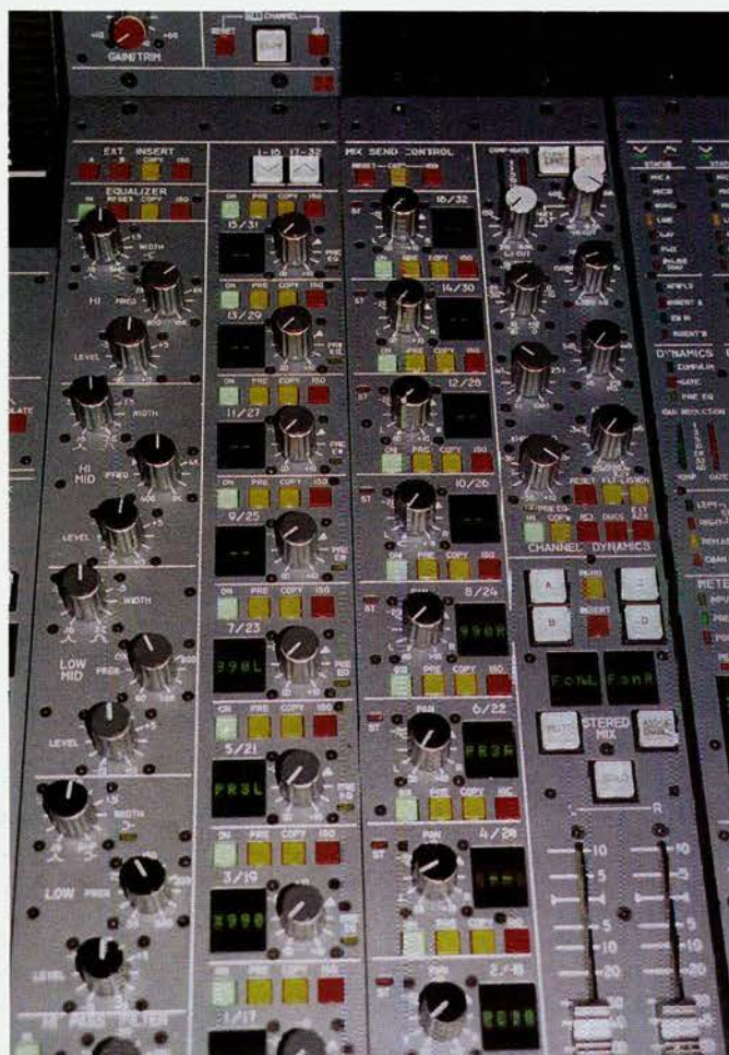
Showconsole's has one master share channel, with fully motorised controls that snap to whatever settings are recalled when you select a channel.
