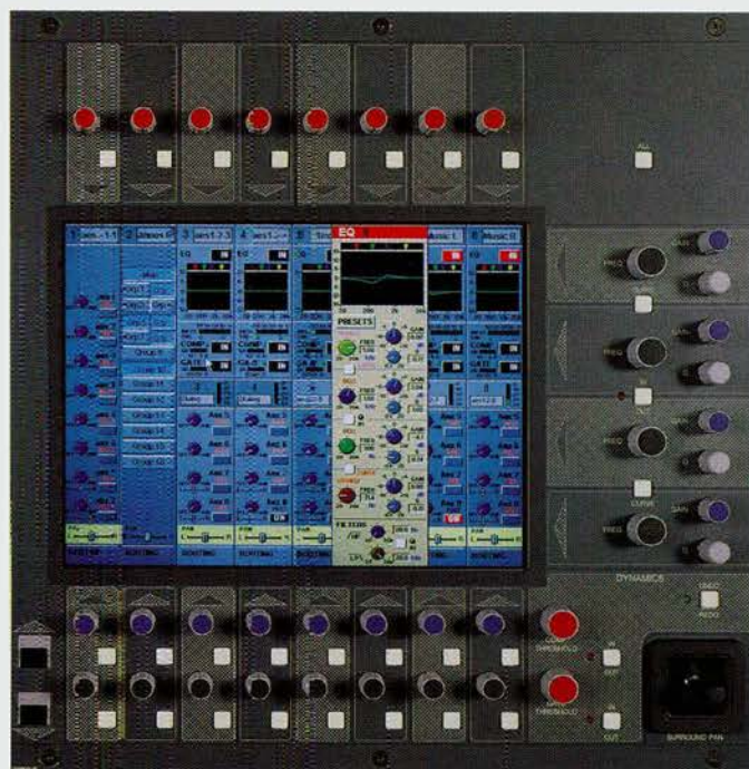
Top of the channel block, showing a detailed EQ screen. The actual EQ rotary controls are those at the right, above the surround panner.
