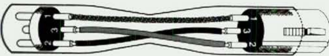
PHASE CHANGE ADAPTOR: PIN #3 ON ONE END CONNECTED TO PIN #2 ON THE OTHER END
