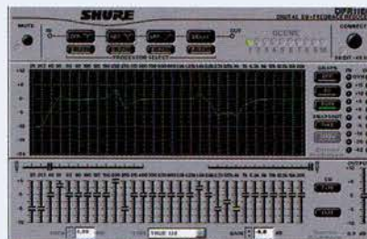
Figure 2: Shure's "True" 1/3 octave equaliser mode. Compare the frequency response curve with Figure 1. This is a "graphic" equaliser!
