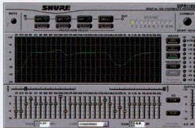
Figure 1: Shure's "Combining" mode equaliser. Compare the frequency response with fader positions. This is not a "graphic" equaliser!
