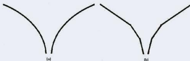
Figure 2: How horns have changed. The exponential horn (a) has largely been replaced by the so called constant directivity horn (b).
