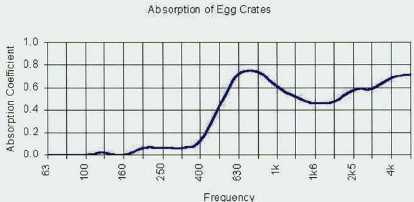
Figure 5: Absorption of egg crates mounted against a hard wall. Don't use them unless you like a muddy, harsh sounding room!
