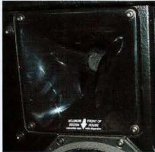
Unique horn topology, allows wider dispersion below the centre axis, and tighter (longer throw) above. May be rotated.
