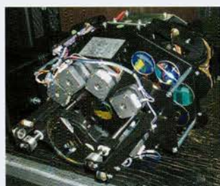
Views of the internal "skeleton" - all of the gobs, prisms, CMY, focus, zoom, the iris and the associated motors for these items are located in this one unit.
