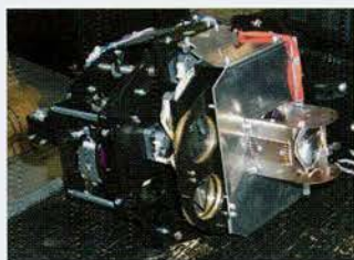
Views of the internal "skeleton" - all of the gobs, prisms, CMY, focus, zoom, the iris and the associated motors for these items are located in this one unit.
