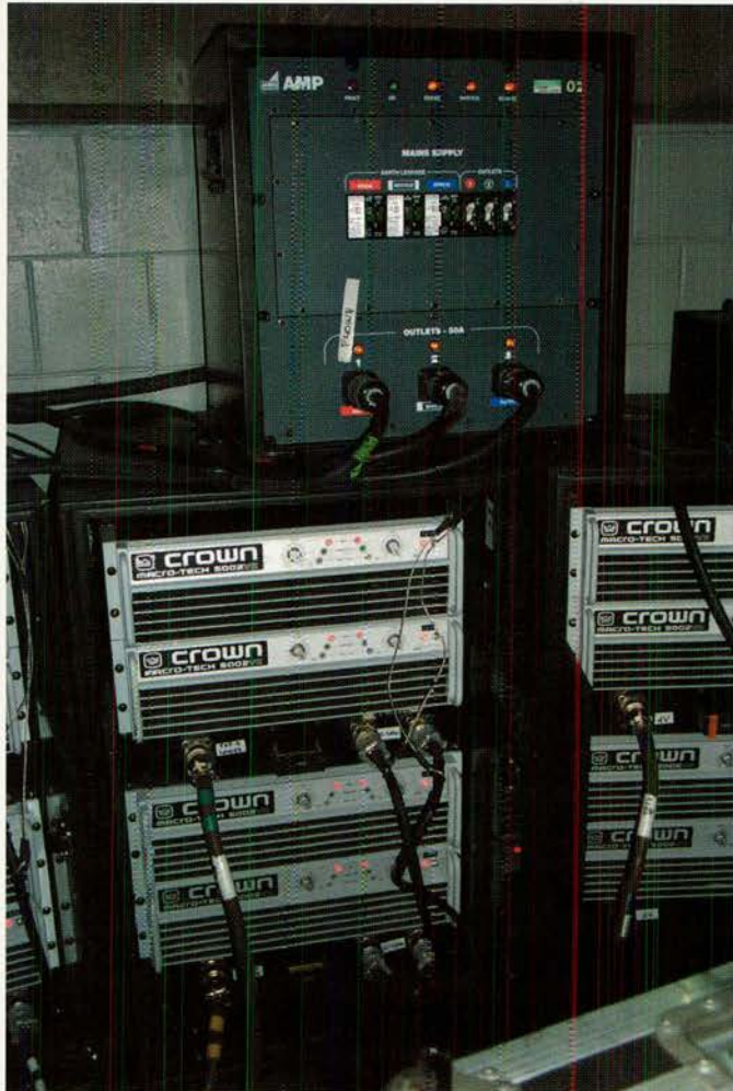
Jands Production Services V-DOSC amp racks are designed to be flown when required. One rack of four amps powers 6 V-DOSC cabinets.
