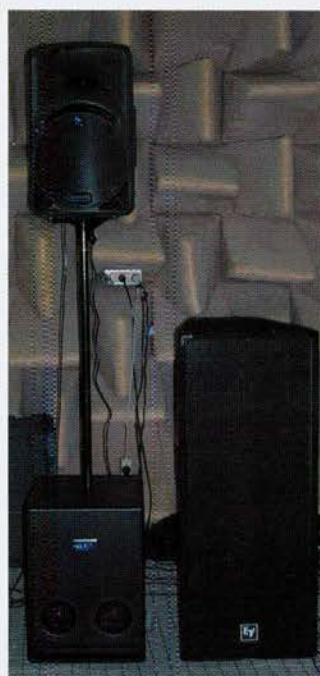
Mackie SRM 450 12" and horn powered box with SRS 1500 single 15" powered sub.
