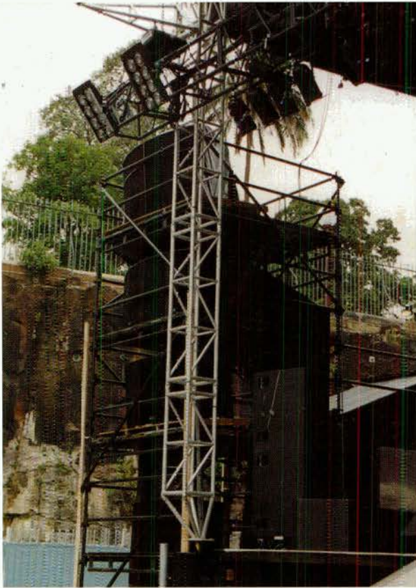
Speakers on scaffold beside stage; 2x MSL-6, 4x DS-4P, 4x MSL-4, 2x CQ-1 and 2x UPA each side.
