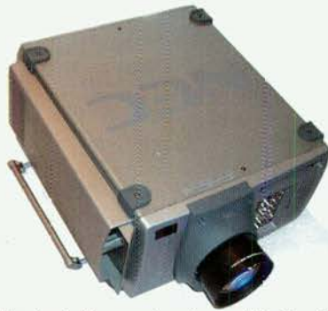
Note the tractable carry handle, and the four 'feet locators' for stacking multiple projectors
