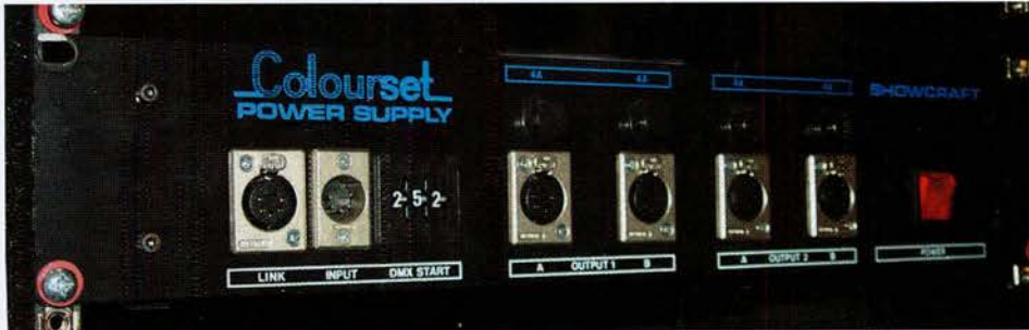
This power supply for Colourset Scrollers uses five pin XLRs for sending power and data to scrollers. Under the new standard, this device could not claim to be compliant with the standard.
