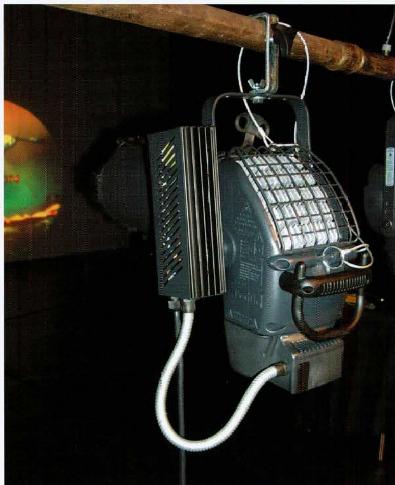
(be.ow) The 80V 1200W Pacific with its electronic power supply. Also note the new heat-sink protection grill
