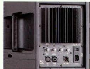
The SxA100 features mic and line level inputs for easy mixing, two-band EQ, and line-level out
