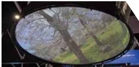
Under the Dome - huge immersive projection three metres across created with a Panasonic PT-RQ22K 21,000 lumen 3 chip DLP with 4K
