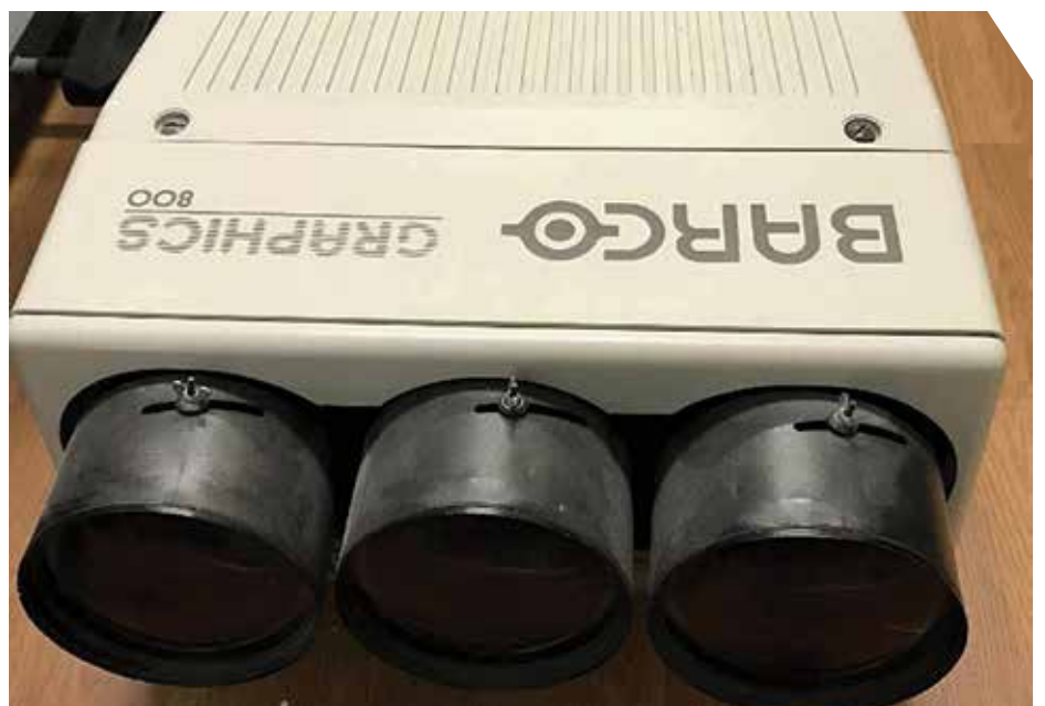
A Barco Graphics 800 CRT data projector. Cost about $35,000 and produced about 800 ANSI Lumens.
