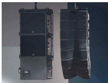
Eight Kiva II enclosures per side flown next to three SB15m subwoofers in cardioid mode minimises low-frequency spill onto the stage.
