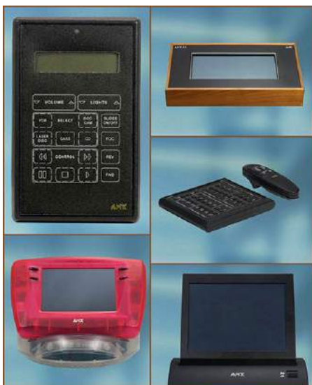
Clockwise from top left: One of the world's first advanced wireless remote controllers. The very first AMX touch panel. An early home theater remote control center. The first tilting AMX touch panel. Translucent colored touch panels.
